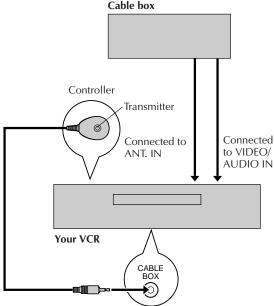
This procedure is required if you receive your TV channels through a cable box (descrambler). The Controller allows the VCR to automatically switch the cable box channel during timer-recording. The Controller is effective for recording shows that have been programmed using VCR Plus+ (\$\mathbb{C}\mathbb{T}\$ pg. 36) or Express Timer Programming (\$\mathbb{C}\mathbb{T}\$ pg. 40).
